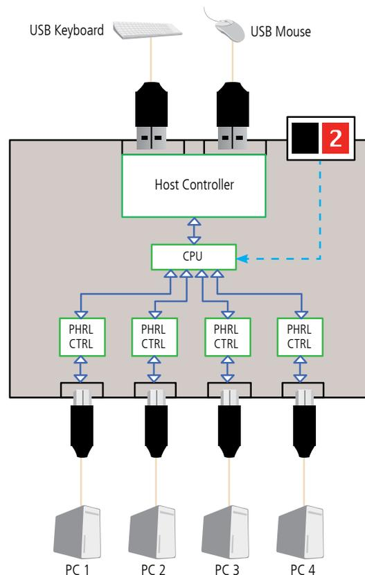
*The inside view of a typical emulated USB switch.*
