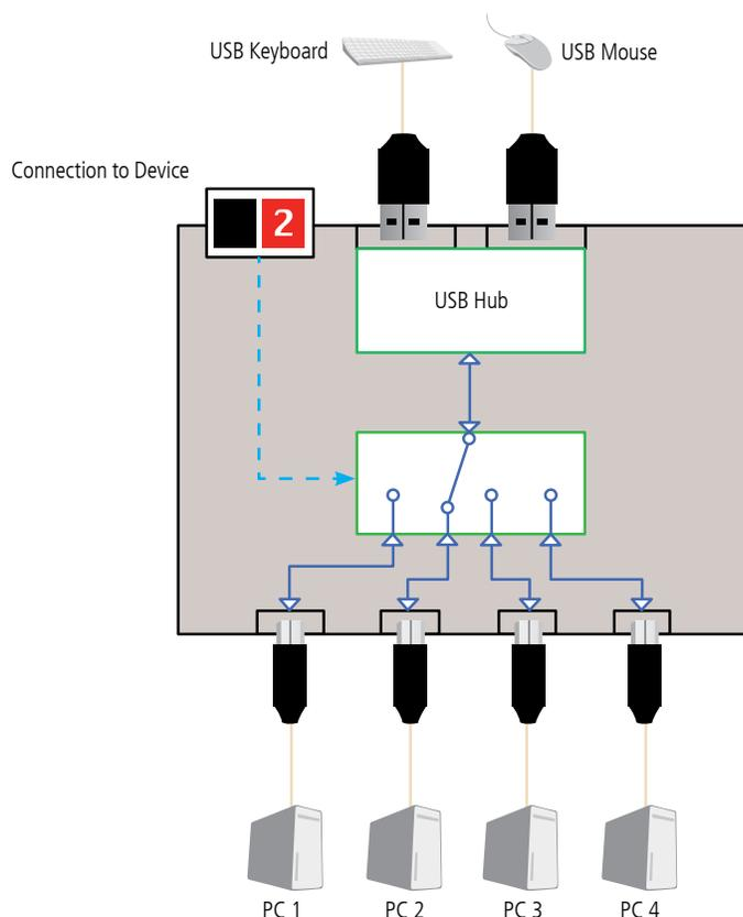
*The inside view of a typical enumerated USB switch. The keyboard and mouse are linked to a hub, which then feeds via a simple electronic switch to the selected computer.*
