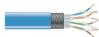
S/FTP: shielded/foiled twisted pair (A braided shield over four individually foil-shielded twisted pairs)
