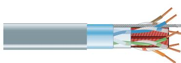
F/UTP: foiled/unshielded twisted pair (An overall foil shield over four unshielded twisted pairs. Shown with rip cord, Mylar™ sheath, and pair separator.)
